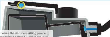
Ensure the silicone is sitting parallel on the hole below it. Hold at eye level to check the position is correct
