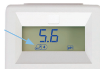
Successful pH 7 and pH 4 calibration
