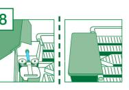
Place lid over the AQUAvalve compartment of the tray and press securely into position
