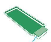
Wet and lay root control sheet on top of capillary matting. The root control sheet can be laid copper side up or down.
